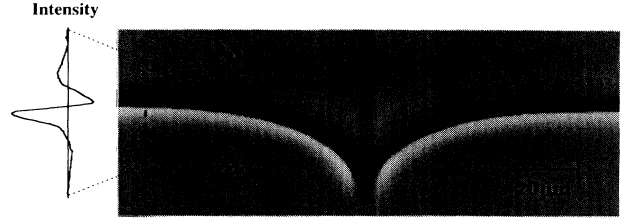
FIG. 5. Measured interface coordinates superimposed on photograph of cusp. X = 0.585 , h = 12.5 \mu\text{m} , phase-contrast microscopy. The vertical graph shows the light-intensity profile perpendicular to the interface.
